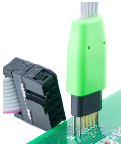
Figure 49 - Tag Connect Header inserted into PCB
