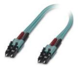
Assembled FO cable, zip cord cable, multi-mode fiberglass 50/125  $\mu$ m, OM3, plug: LC/LC, degree of protection: IP20, for installation in cable ducts or control cabinets, length: 2 m
