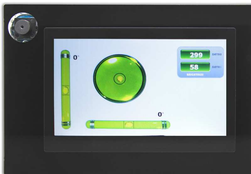
Figure 4-10 Digital Accelerometer demonstration
