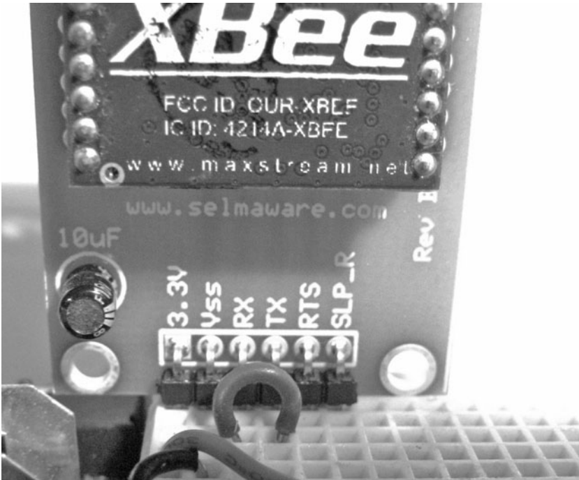
Figure 5-8 Remote XBee connections for loop-back.
